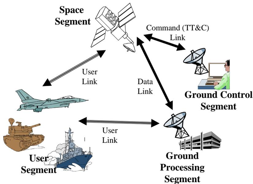
**Figure 2. Segments and Links of a Space System**
