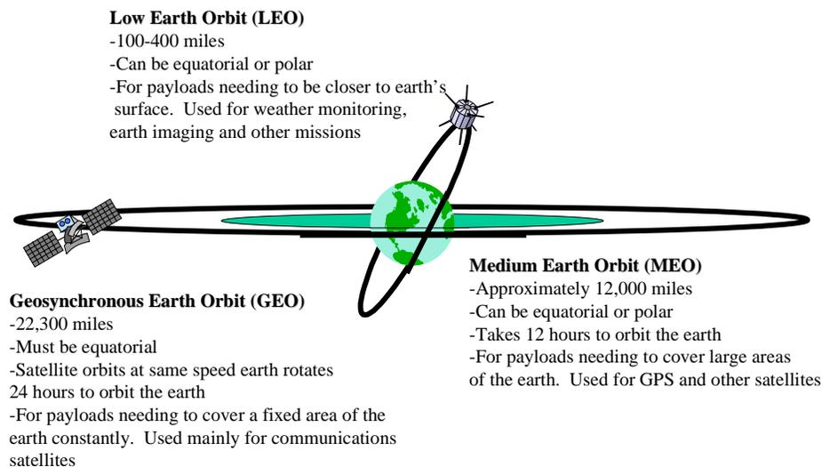
**Figure 4. Three Most Common Types of Satellite Orbits**
