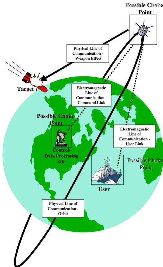
**Figure 5. Space Choke Points and Lines of Communication**
