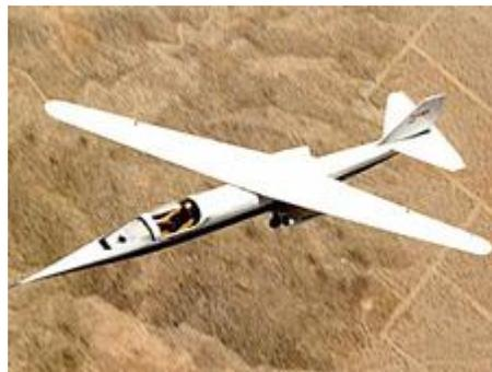
**Figure 9: NASA AD-1 Oblique Wing Demonstrator<sup>40</sup>**
