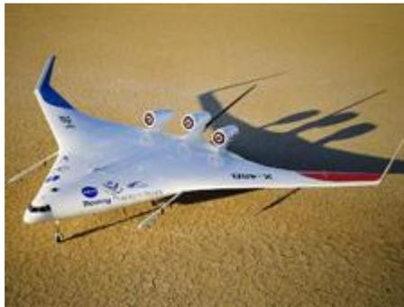
**Figure 10: Boeing's X-48 Blended Wing-Body Technology Demonstrator<sup>43</sup>**
