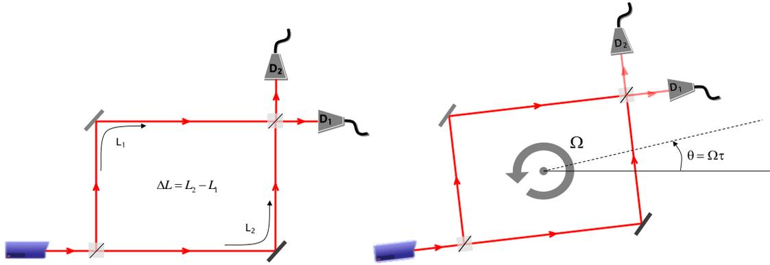
Figure 1: Basic set-up of an optical interferometer to measure rotation.<sup>16</sup>
