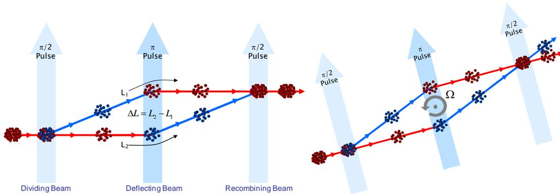
Figure 2: Basic principle of an atomic interferometer to measure rotation.<sup>18</sup>
