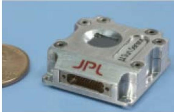
**Figure 4** Miniaturized sun sensor developed by NASA's Jet Propulsion Laboratory and used as part of the KUTESAT-2 mission. (Reprinted from Sorensen et al, "KUTESAT-2, a Student Nanosatellite Mission for Testing Rapid-Response Small Satellite Technologies in Low Earth Orbit." In *AIAA 3rd Responsive Space Conference*. Los Angeles, CA: AIAA, 2005.)
