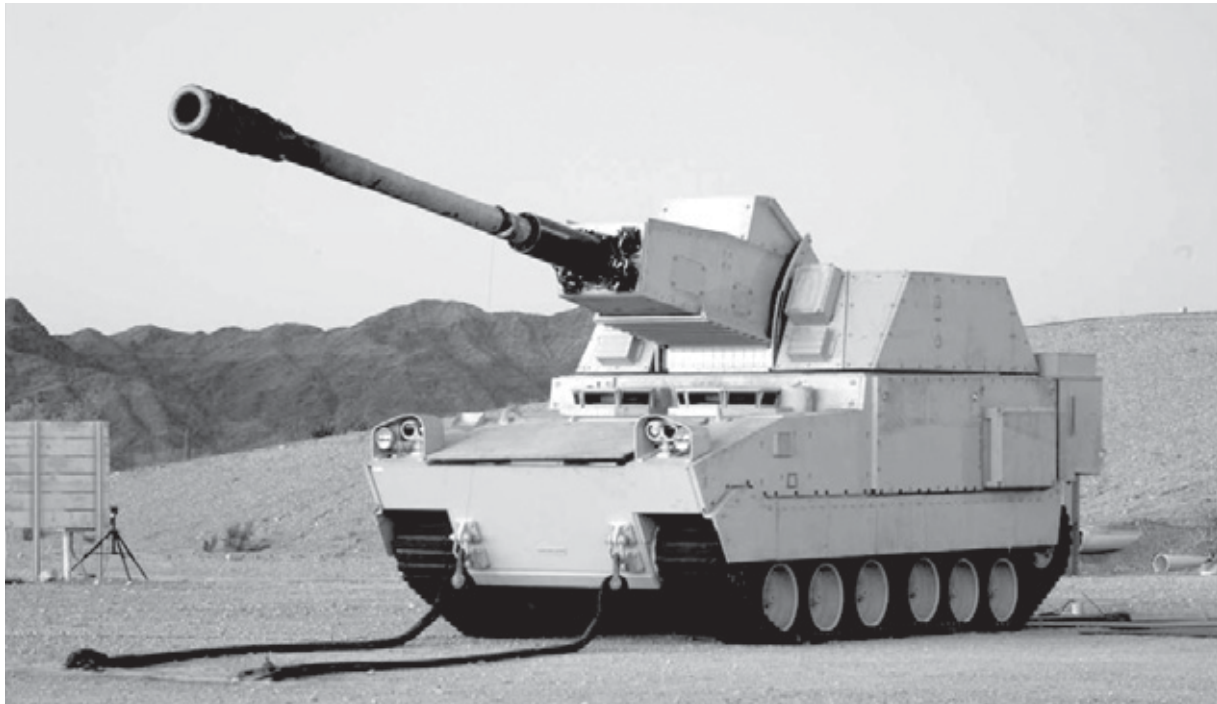
The XM1203 Non-Line-of-Sight Cannon was a mobile 155-mm cannon intended to provide improved responsiveness and lethality to the unit of action commander as part of the U.S. Army's Future Combat Systems project, Yuma, AZ, 2009.
