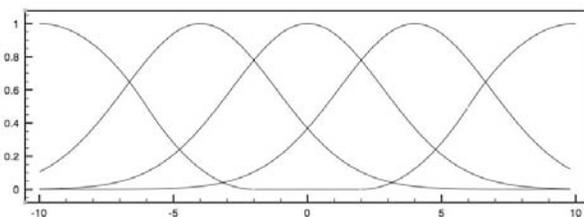
**Figure 4.** Fuzzification of a real variable over a range of -10 to 10.
