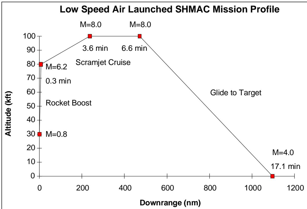
Figure 3-5. Low Speed Air Launched SHMAC Mission Profile.
