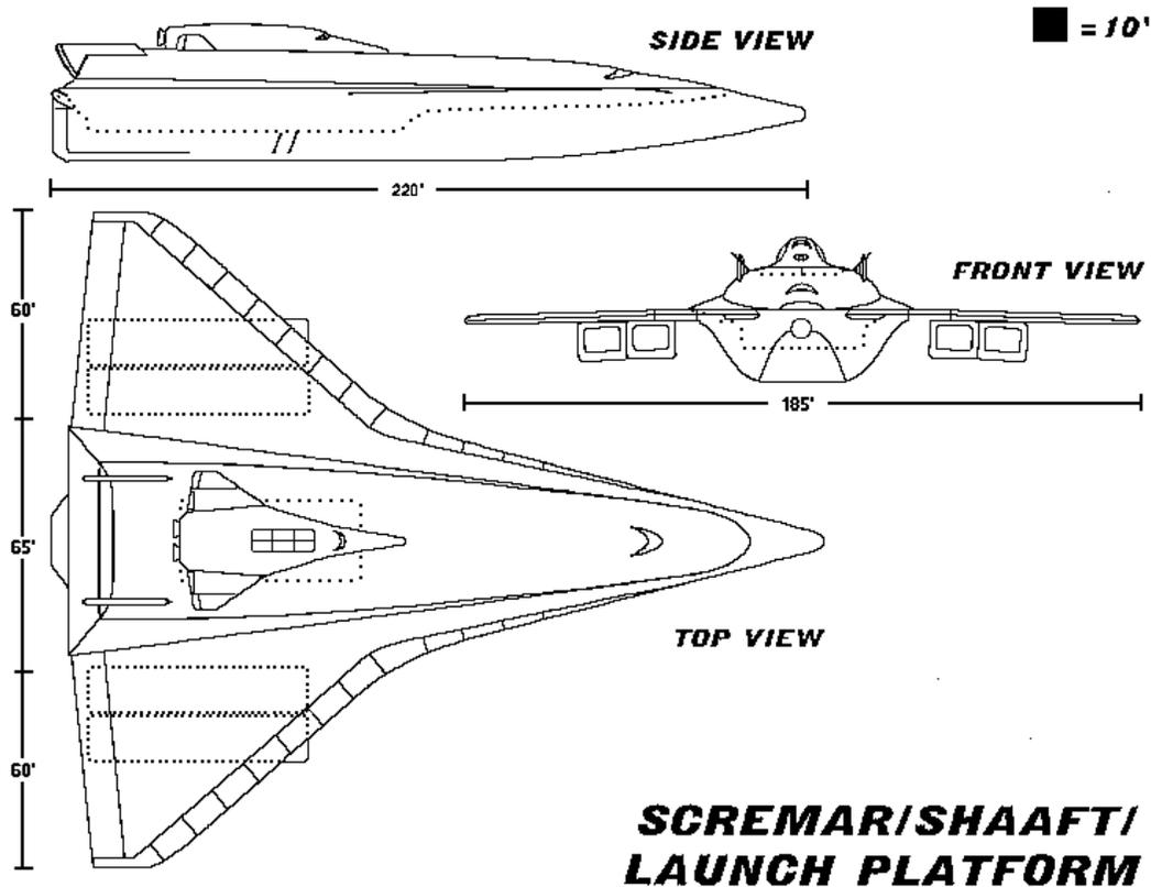
**Figure 1-4. Schematic of Mated S<sup>3</sup> Platform (with SCREMAR).**
