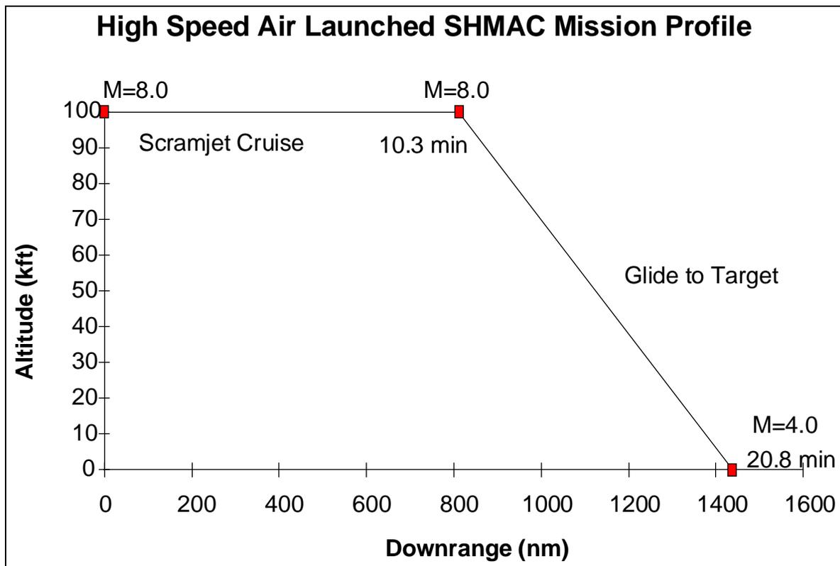
Figure 3-4. High Speed Air Launched SHMAC Mission Profile.
