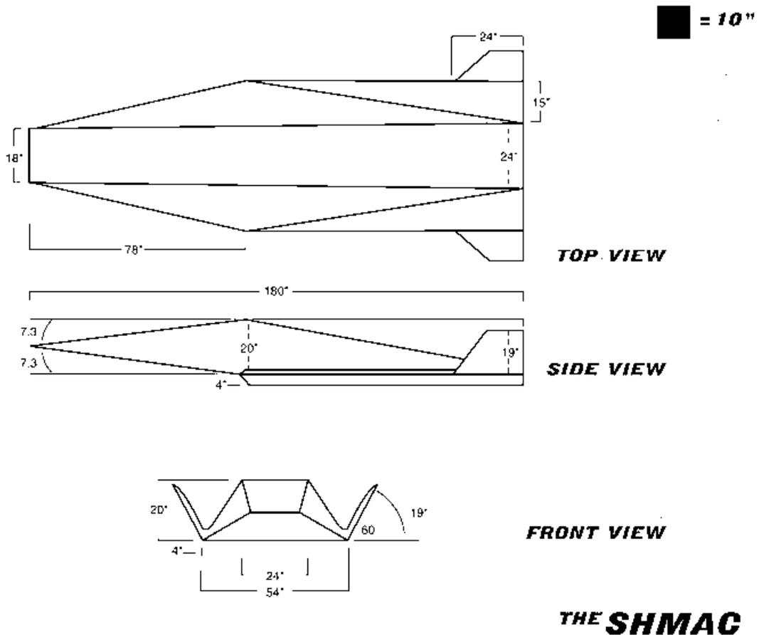
**Figure 3-2. Standoff Hypersonic Missile with Attack Capability (SHMAC).**
