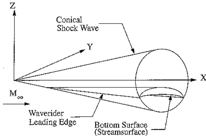
**Figure 2-2. Conically Derived Waverider.**
